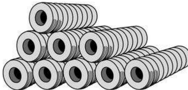
FIGURE A.3.9.4.9(e) Palletized Portable Tire Rack, On-Side Storage Arrangement (Banded or Unbanded).
