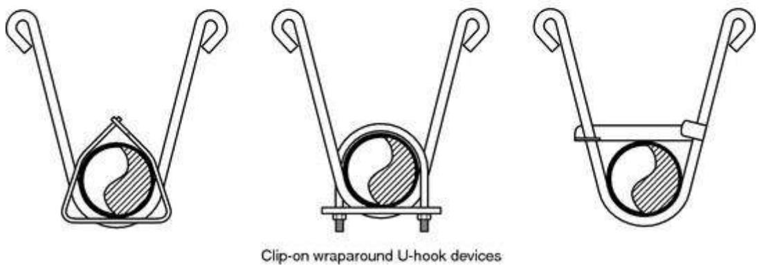
FIGURE A.9.2.3.4(b) Examples of Acceptable Hangers for End-of-Line (or Armover) Pendant Sprinklers.
